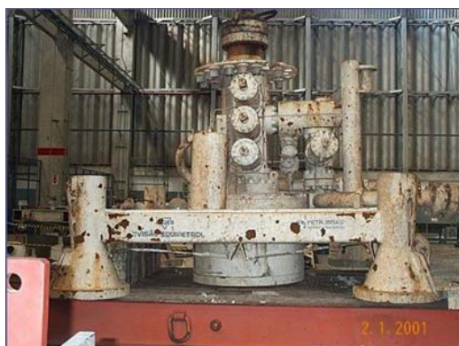
Figure 8. Christmas Tree - Subsea Equipment (After 20 years submerge) (Internet: www.cortecvci.com/cortec-corrosion-solutions-available-around-the-globe )
